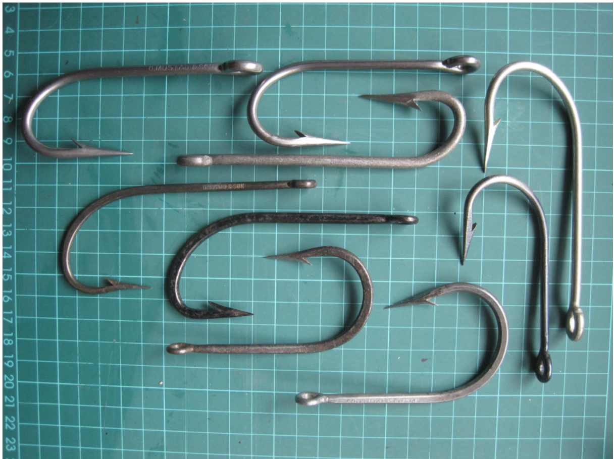
Hooks seen and used. Top - Mustad Kirby Kendal 4x strong sizes 11/0 and 12/0; underneath is a Mustad 4480 1" (now called 10/0) Shark Hook, then a 12/0 Mustad O'Shaughnessy 3406 above a 4" Hardy Limerick (as used on tunny - a rare hook) and under that are two Mustad Sea Master 7699 10/0 and 11/0. On the right is a 14/0 Mustad Best Kirby tinned 3138 above a blued Mustad Kirby 2320 size 1. These last two are typical of the commercial hooks pressed in to use at times.
