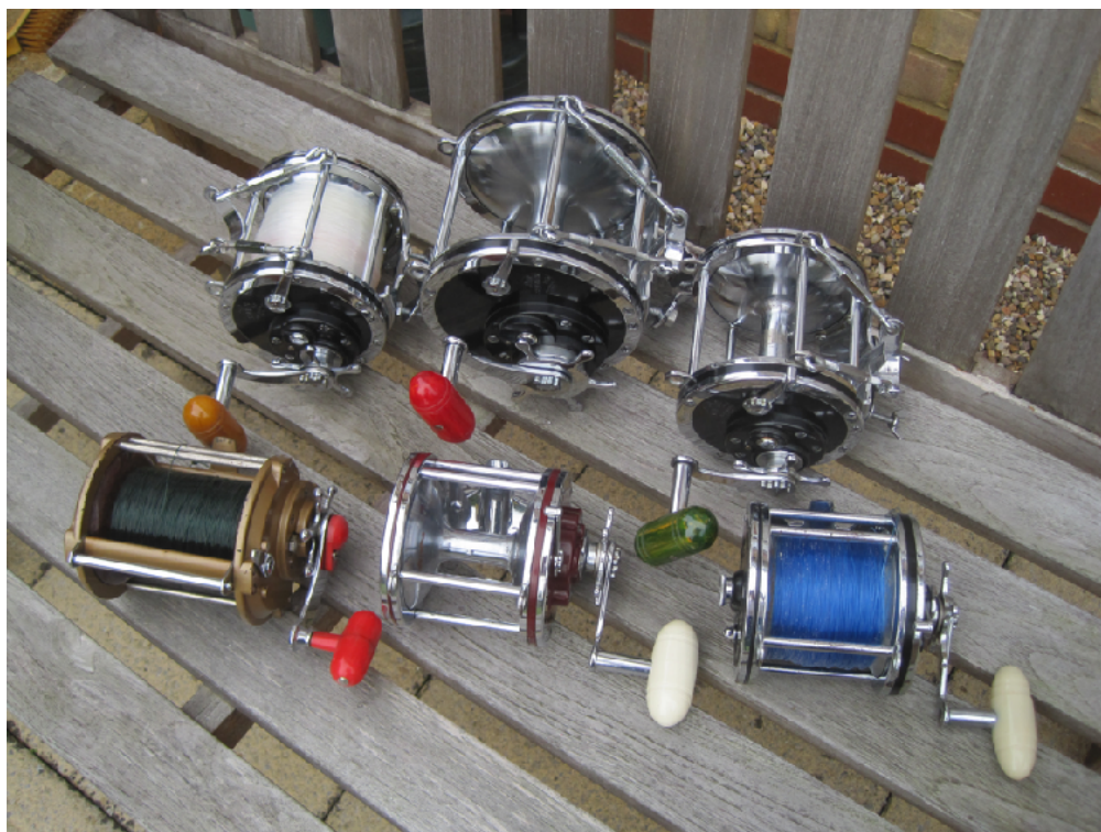
A 12/0 Senator flanked by two 9/0. In front is a Tatler V on the left, a 6/0 Senator on the right and the red plate 6/0 in between. The "posh" red plate 6/0 had ball bearings and an upgraded drag compared with the standard black plate 6/0
